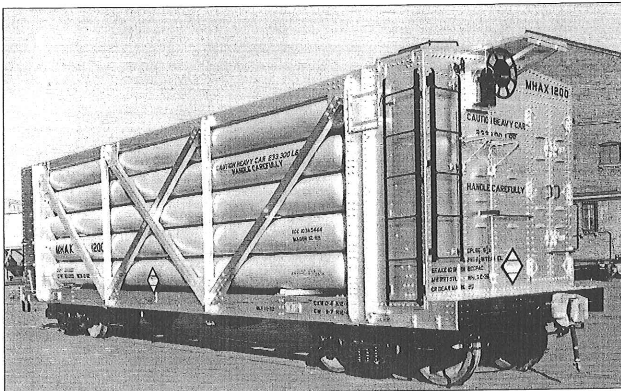
Eighth Generation: 30-Tube Car Built by Magor; May 1962 1197-1221 (Painted all aluminum and these were the last cars built)
